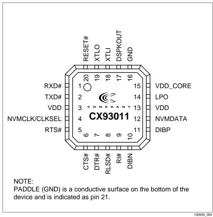
Figure 3-2. CX93011 Modem 20-Pin QFN Pin Signals
