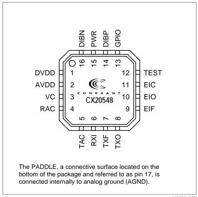
Figure 3-4. CX20548 LSD 16-Pin QFN Pin Signals
